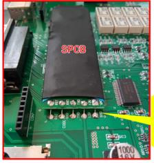
Step1. Remove SPCB Attention: Do not damage the PCB pad
