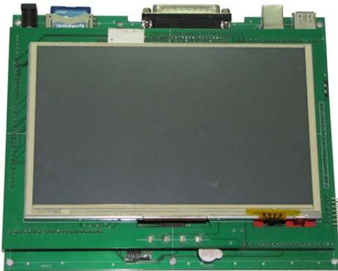
Seperate the two PCBs connected together as shown below.
