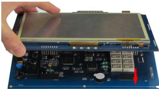
Completed construction of new PCB and screen should look like below.
