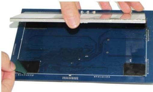
Join the two PCB's together.
