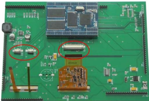
Carefully remove the screen from the top PCB as shown below.
