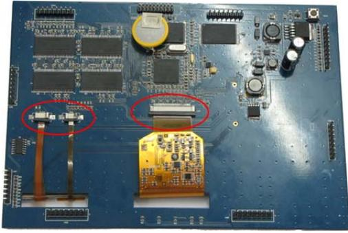
Stick the screen to the PCB using the double-sided tape as shown below.
