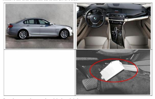
Open the case, and remove the unit in the red circle.
