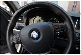
Ignition on. Press BC button on end of steering wheel stalk and MODE button on steering wheel at the same time to switch on/off counting.
