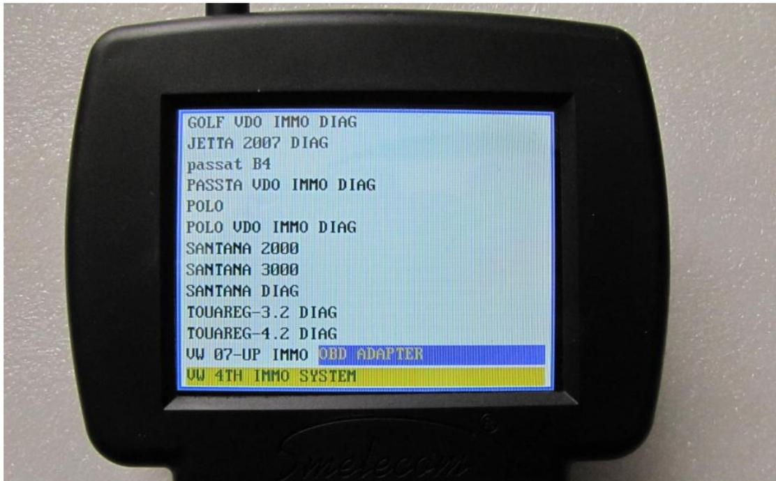
Step 4. Choose "IMMO SYSTEM (NEC)" or "IMMO SYSTEM (CDC)", if you do not know which IMMO system the car is then choose "AUTO-DETECTION OF IMMO SYSTEM", it will detect which kind of the IMMO system is used in the car. If both are not, just choose the option "IMMO SYSTEM(1M80F)". And for some latest VW cars, it has NEC+24C64 in the car, now you should choose IMMO SYSTEM(NEC+24C64). If you want to do REMOTE ADAPTION, please choose the corresponding option 1 or 2, for NEC type or CDC type.
