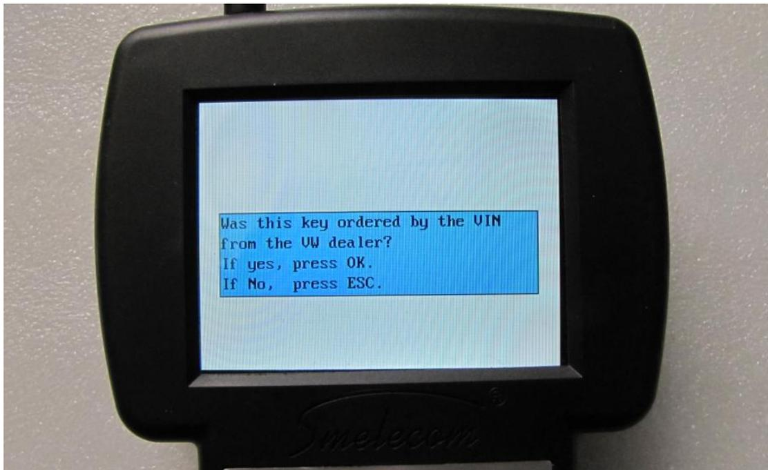
**KEY ADAPTION** In step 7, if you press “ok”, you will come to the KEY ADAPTION menu. In this menu there are two selections “Add a new key” and “ Register the keys”. “Add a new key” is to add a new key to the car and keep all the original keys for the car. “ Register the keys” is to register all keys to the car, so you must keep all keys available to hand.
