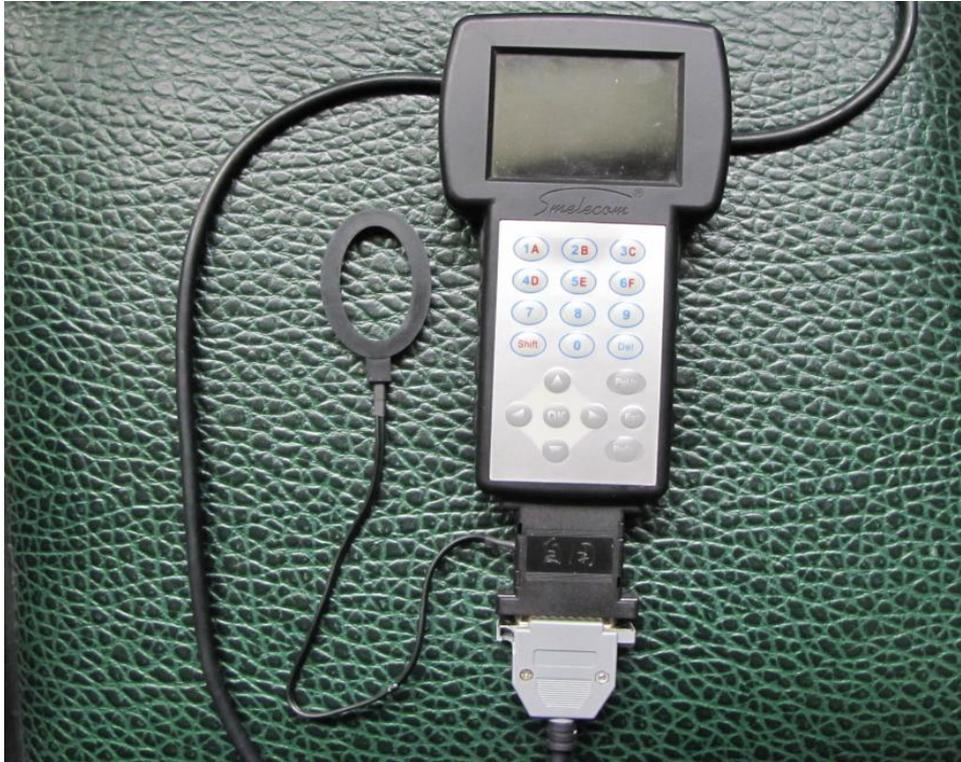
Step 2. Connect OBD adapter to the diagnostic socket of the car, choose "IMMO" from the main menu,
