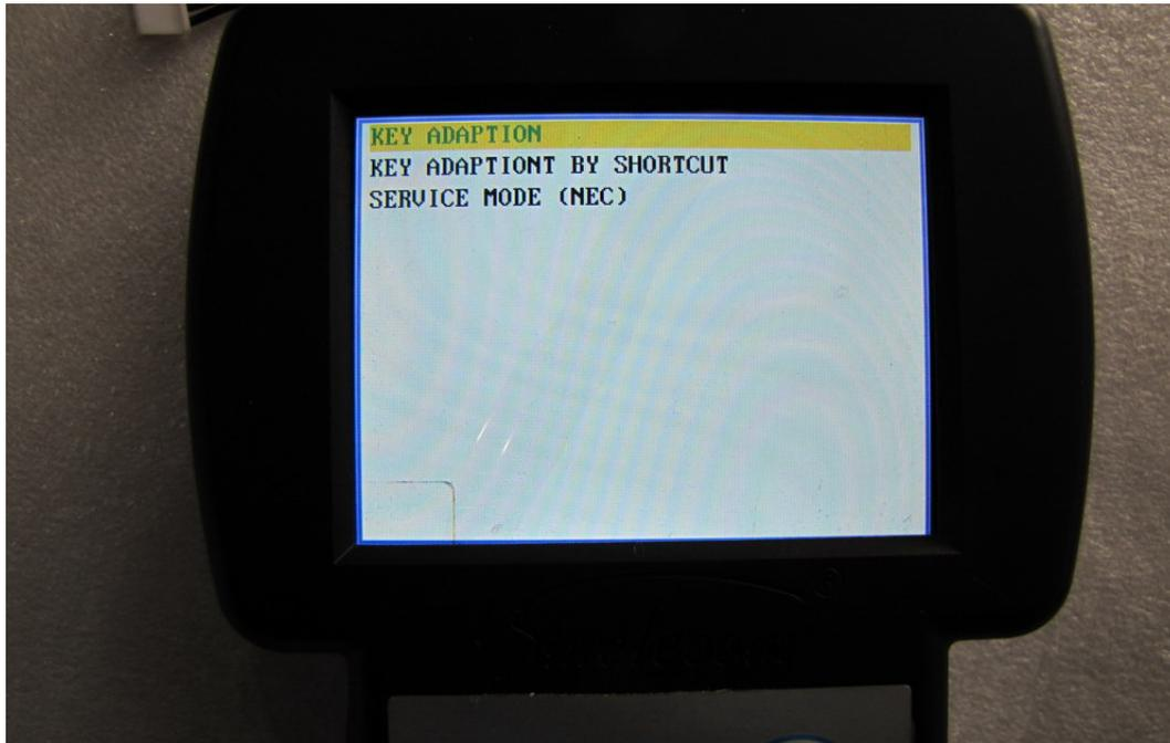
Step 6. In this step, you need to turn on the ignition, normally you should keep at least 2 keys available to hand, one is to turn on the ignition, the others are to be adapted to the car. Press “OK” to continue.
