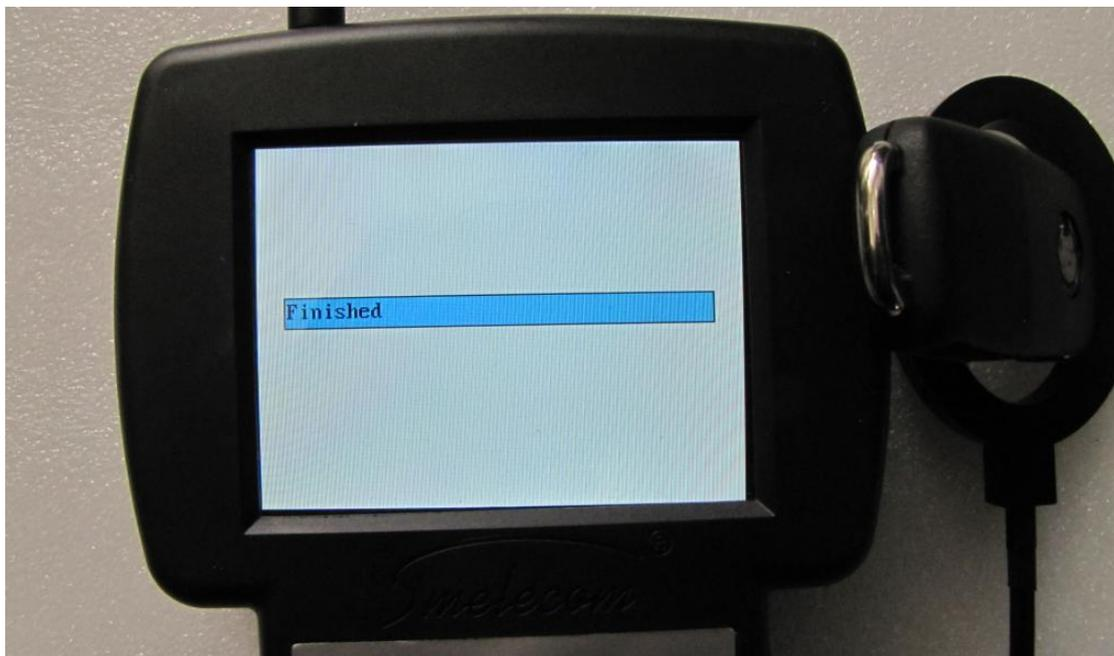
**Register the keys:** This function will register all the keys to the car, so you must keep all keys available to hand (such as if you leave one key at home, after this function is finished, the key at home will not work on this car), and then go on step by step according to what the tool tells you to do. When finished you can start the car with any of the keys registered to this car.
