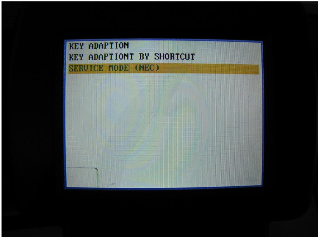
**For the NEC type IMMO system, sometimes the software will display “SERVICE MODE NEEDED”, you should then remove the 24C32 eeprom from the odometer, place it in the eeprom adapter socket and select “SERVICE MODE” . After this program completes, install the 24C32 eeprom back into the odometer, aslo install odometer back into the car , and continue to the next step by OBD.**
