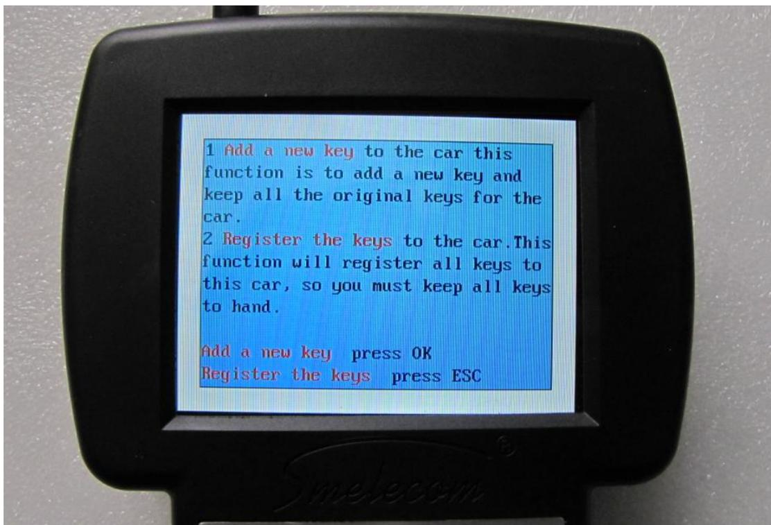
**Add a new key:** In this step you can delete all the keys from the car; press “OK” to add a new key, press “ESC” to delete all keys. Normally you should press “OK” to add a new key. After about 5 minutes, it will show “finished”, this means the new key is successfully adapted to the car. You can start the car by the key.
