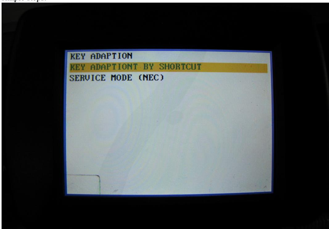
**IMPORTANT NOTE:** when making key adaption or writing key, you must put the transponder in the transponder adapter correctly, otherwise the tool cannot read ID from the key. Then you need to modify the position of the transponder; the transponder should be inside the ellipse and near the ellipse enough. Sometimes you put a key inside the ellipse and near the ellipse, but in fact the transponder inside the key is not inside the ellipse or near the ellipse!!
